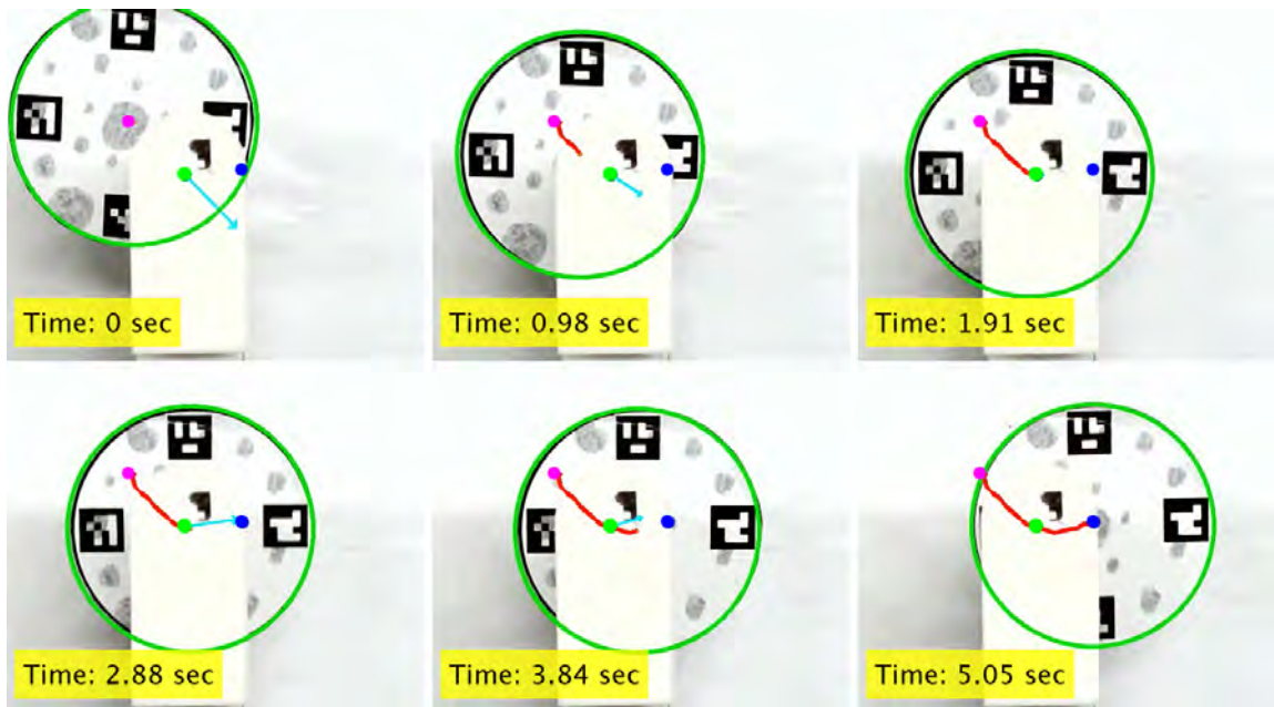
Figure 5.7: Manipulating the COM of a disk from an initial position (magenta marker) to a goal position (blue marker) through the origin (green marker). The disk reached the goal with an accuracy of 2 mm error and 4.39^\circ orientation change.
