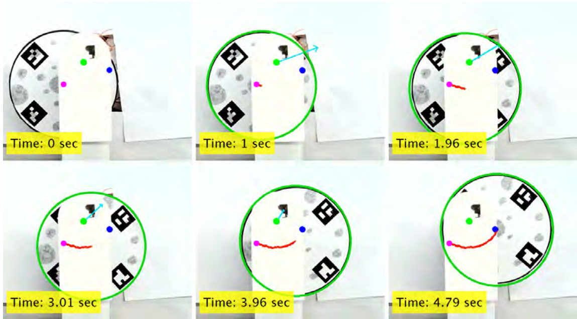
Figure 5.6: Manipulating the COM of a disk from an initial position (magenta marker) to a goal position (blue marker). The disk reached the goal with an accuracy of 1.93 mm error and 9.94^\circ orientation change.
